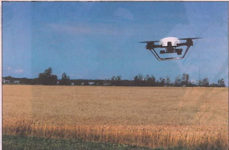
Unmanned aircraft can be used to monitor agriculture. For example, a drone with a spectral camera can detect stress levels in plants due to a lack of water or nitrogen. - Photo courtesy of SkySquirrel Technologies
